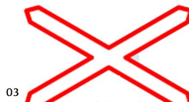
03 Level Crossing Without Gate Barrier
